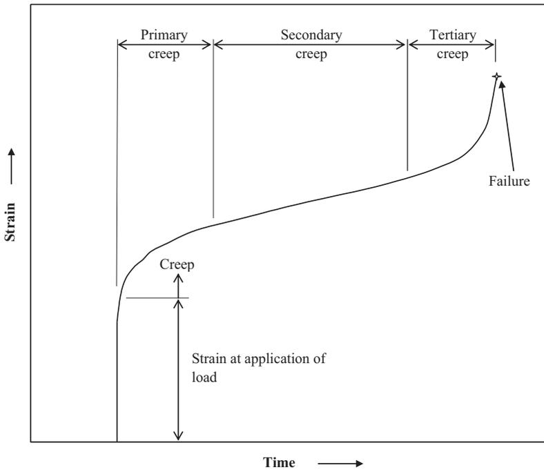
**Figure 2.2** General form of the strain–time curve for material undergoing creep leading to failure [1].
