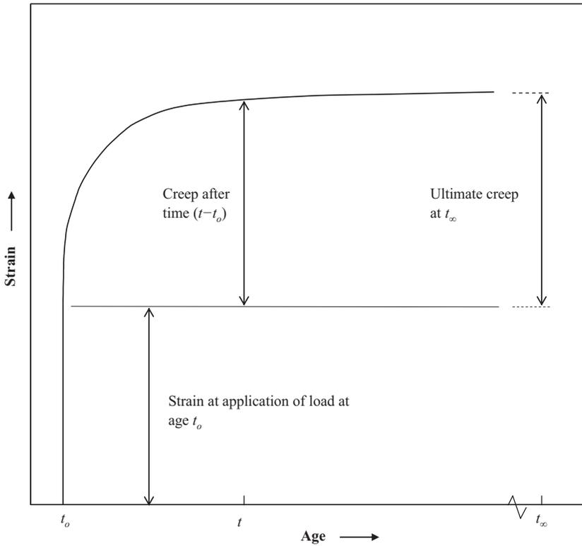
**Figure 2.3** General form of the strain–time curve for concrete and masonry subjected to normal levels of sustained stress.
