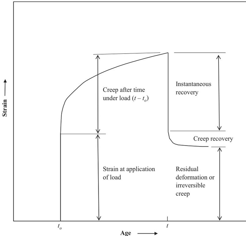
**Figure 2.6** Instantaneous and creep recoveries after concrete or masonry has been subjected to load from age  $t_0$  and unloaded at age  $t$  [1].
