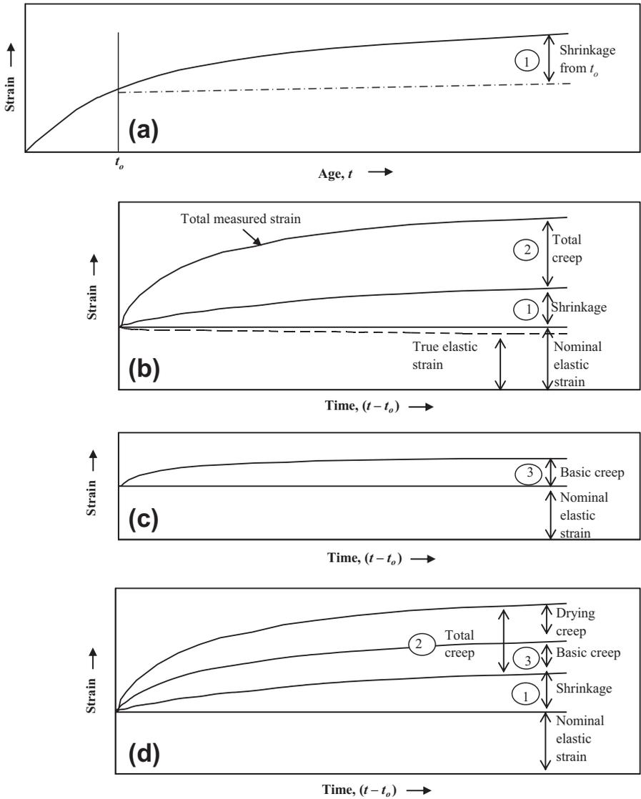
**Figure 2.4** Definition of terms used for elastic strain and creep [1]. (a) Shrinkage of a load-free control specimen. (b) Total measured strain of a loaded and drying specimen. (c) Strain of a loaded and sealed specimen. (d) Components of strain of a loaded and drying specimen.
