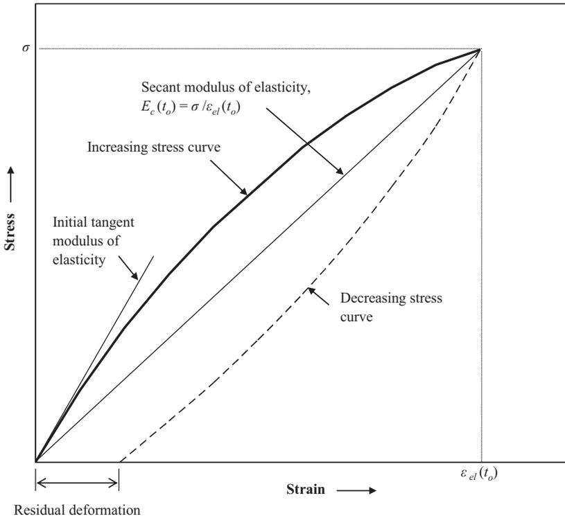
**Figure 2.5** Generalized enlarged stress–strain curve for concrete and masonry [1].
